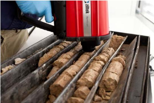
RemScan is used to measure the concentration of oil on the surface of the soil enabling the user to quickly delineate the contaminated area. Depth profiles can be measured by taking a drill core, laying the core out and using RemScan to directly measure the hydrocarbon concentration at various points (depths) along the core.
